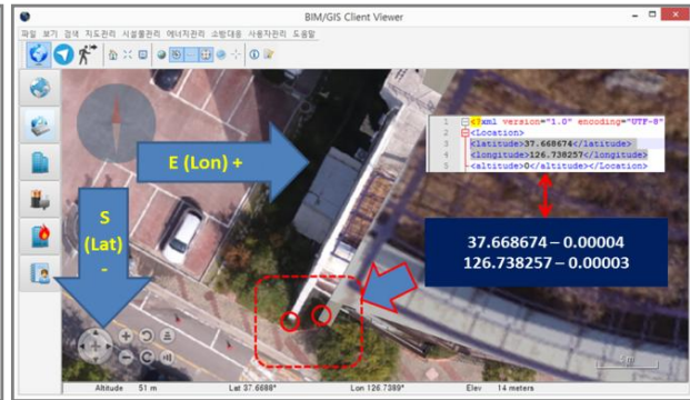
Figure 8: Location correction to solve the error
