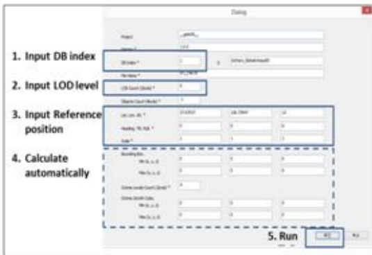
Figure 7: Absolute coordinate mapping to IFC data
