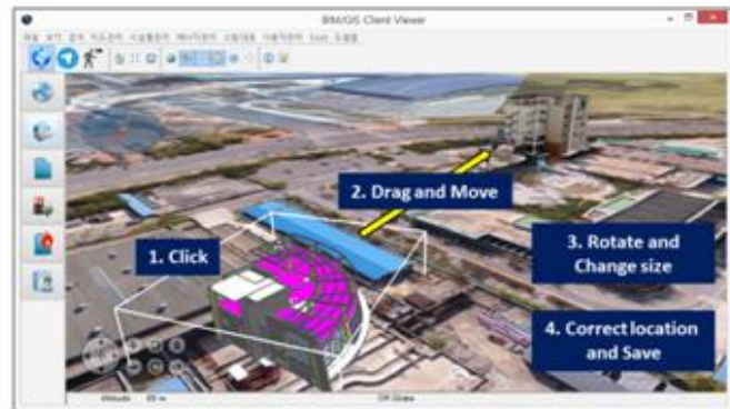
Figure 8: Location correction between BIM/GIS data and 3D texturing data
